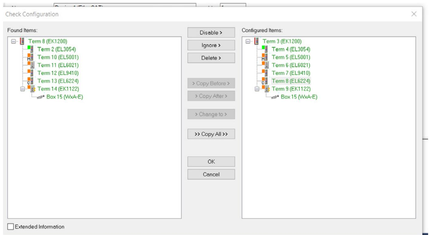
The WxA-E device should appear in the EtherCAT device list. Compile and download this configuration to your PLC. The control window allows you to view the real-time process data and read/write the dictionary objects via SDO protocol.
