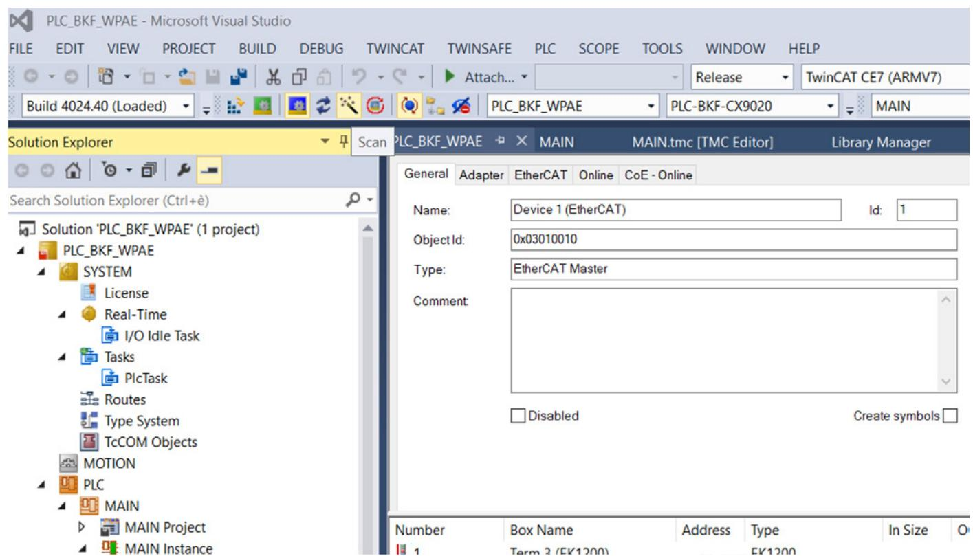
The TwinCAT software shows you the device found after scanning. Select the WxA-E and copy the device into your project.
