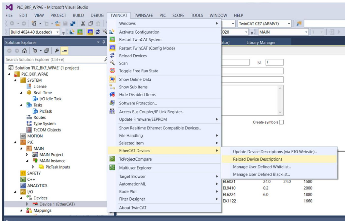
To add the WxA-E sensor to your project, put the Beckhoff PLC into configuration mode, select the EtherCAT master device and click on the Scan button.
